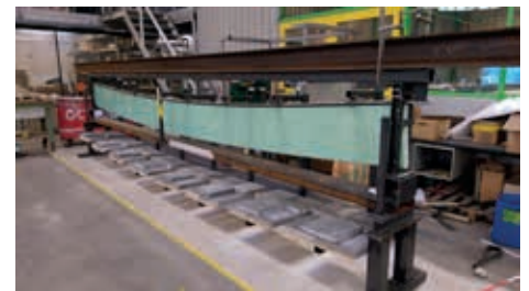
Figure 13: Proof of the pudding: Zappi glass fin fully broken without yielding for 4 weeks
