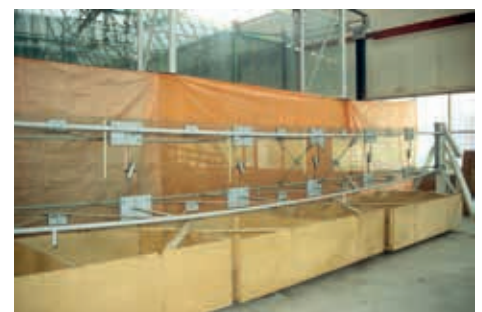
Figure 2: Zappi-fin was kept 4 weeks fully loaded and fully broken without yielding
